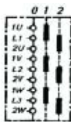
▲ ▲ 2 Speed, 2 Winding (OFF-LOW-HIGH)
