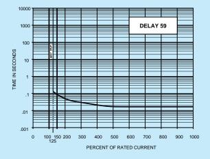
DC/50/60Hz Delay Curves (typ) (Multi-Frequency)
