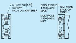
Note: Tolerance ± .031 [.79] Angles: ±5° unless noted. Dimensions in brackets [] are millimeters.
